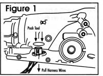
2. The Harness Removal Tool fits a standard bushing driver handle and can be used while harness is in
